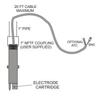
ELECTRODE HOUSING WITHOUT PREAMP SUBMERSION MOUNT
